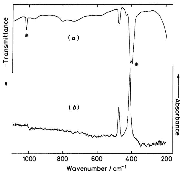
**Figure 1.** (a) Typical i.r. spectrum obtained after deposition of  $\text{MoCl}_5$  in a nitrogen matrix. The features denoted \* are due to  $\text{MoOCl}_4$ . (b) Difference spectrum obtained from consecutive spray-ons at a later stage of sample deposition
