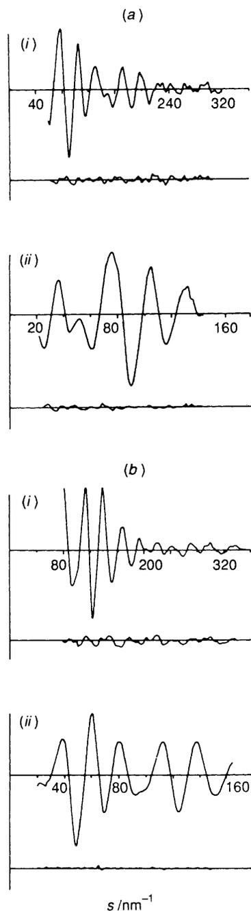
**Figure 4.** Experimental and final difference molecular-scattering intensity curves: (a)  $[\text{Me}_2\text{GaH}]_2$  with nozzle-to-plate distances (i) 128.4 and (ii) 285.4 mm; (b)  $[\text{Me}_2\text{GaCl}]_2$  with nozzle-to-plate distances (i) 98.4 and (ii) 255.8 mm
