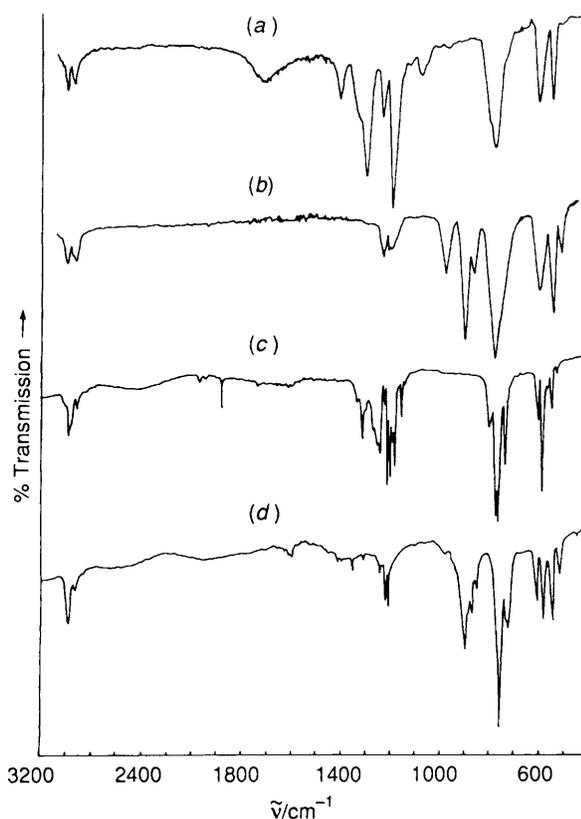
**Figure 1.** I.r. spectra in the region 400–3200  $\text{cm}^{-1}$ : (a)  $[\text{Me}_2\text{GaH}]_n$  vapour, pressure *ca.* 1 mmHg, 290 K; (b)  $[\text{Me}_2\text{GaD}]_n$  vapour, pressure *ca.* 1 mmHg, 290 K; (c)  $[\text{Me}_2\text{GaH}]_n$  vapour isolated in an argon matrix at *ca.* 20 K (argon:gallane = *ca.* 500:1); and (d)  $[\text{Me}_2\text{GaD}]_n$  vapour isolated in an argon matrix at *ca.* 20 K (argon:gallane = *ca.* 500:1)
