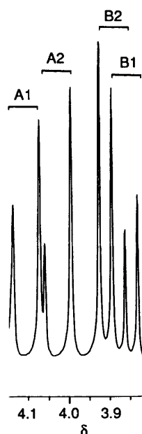
Fig. 8 ^1\text{H} NMR (270 MHz, \text{D}_2\text{O} ) spectrum of -\text{NCH}_2\text{CO}_2- groups in [\text{Zr}(\text{egta})]
