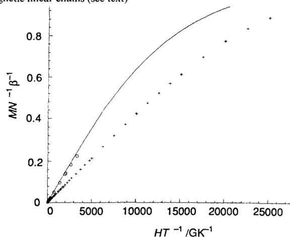
Fig. 3 Magnetization isotherms at 15 K (O) and 2 K (+) up to 51 kG for  $[\{\text{CuL}(\mu\text{-NCO})\}_n][\text{ClO}_4]_n$ . The solid line shows the result obtained by applying the Brillouin formula with  $S = \frac{1}{2}$  and  $g = 2.11$
