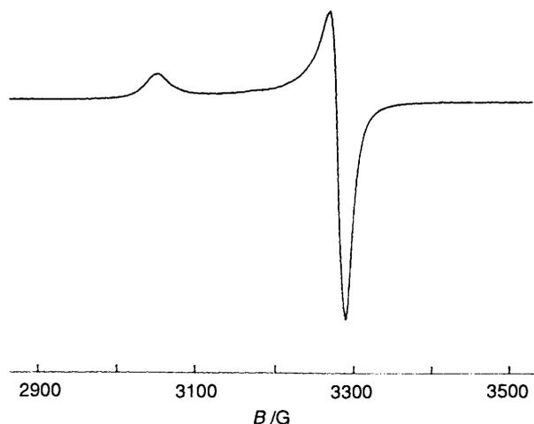
Fig. 4 The ESR spectrum (X-band) of a polycrystalline sample of  $[\{\text{CuL}(\mu\text{-NCO})\}_n][\text{ClO}_4]_n$  at 77 K
