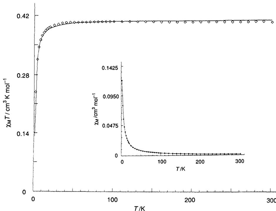
Fig. 2 Magnetic susceptibility plots of a polycrystalline sample of  $[\{\text{CuL}(\mu\text{-NCO})\}_n][\text{ClO}_4]_n$ , solid line shows the best fit using the expression for the magnetic susceptibility of isotropically coupled  $S = \frac{1}{2}$  ions in antiferromagnetic linear chains (see text)
