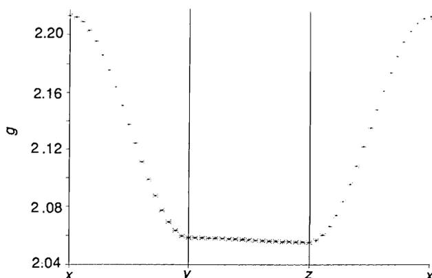
Fig. 5 Angular dependence of  $g$  for  $[\{\text{CuL}(\mu\text{-NCO})\}_n][\text{ClO}_4]_n$  rotated about the three orthogonal axes  $a$ - $c$
