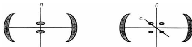
Fig. 1 Schematic representation of the diffraction pattern of a single domain of the nematic phase; the pattern is symmetrical about the director ( n ). Left, usual nematic diffraction pattern; right, nematic with local smectic C ordering as shown by the four spots at small angles (see text)
