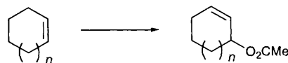
Scheme 2 n = 1, 3 or 7 . Conditions: compound 3 + \text{Cu}(\text{NO}_3)_2 \cdot 3\text{H}_2\text{O} , \text{Na}_2\text{S}_2\text{O}_8 , molecular sieves (3 \text{\AA} ), \text{MeCO}_2\text{H} , room temperature
