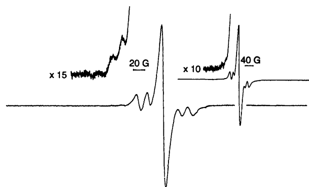
Fig. 6 The EPR spectrum of [Mo 2 (cp) 2 (μ-SMe) 3 (μ-Cl)] ++ in CH 2 Cl 2 at -50 °C showing part of the six- and 11-line patterns. Insert: EPR spectrum of [Mo 2 (cp) 2 (μ-SMe) 4 ] ++ in CH 2 Cl 2 at -50 °C
