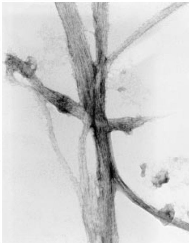
Fig. 13 Transmission electron microscopy image (heavy-metal negative staining methodology) of poly(phenol–formaldehyde) mesofibre bundles templated by mesoporous silica molds. The diameter of the individual fibres constituting the bundles is about 30 Å
