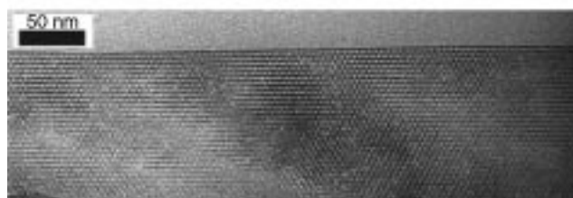
Fig. 9 Scanning electron microscopy (top) and TEM (bottom) images of a free-standing mesoporous silica film grown at the air-water interface
