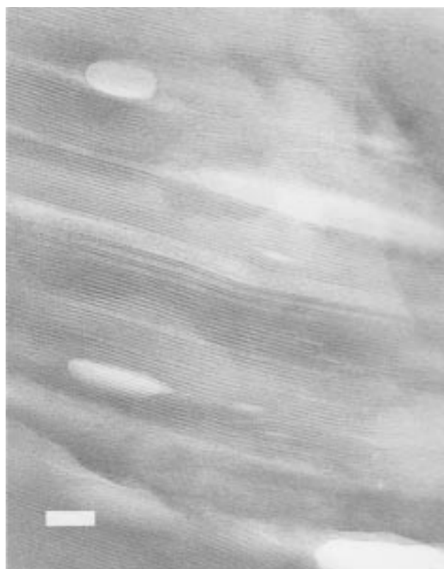
Fig. 2 Transmission electron microscopy image showing the meso-lamellar structure of the aluminophosphate morphologies (scale bar: 30 nm)
