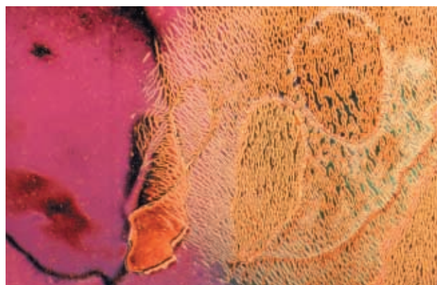
Fig. 8 The transition between the nematic and smectic C phase of compound 16 at 236 °C on cooling showing the classic 'fingerprint' texture.
