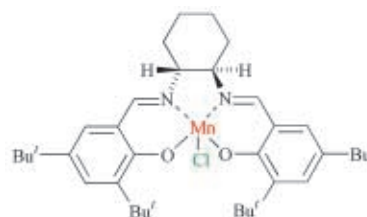
Fig. 8 One of the molecules devised by E. N. Jacobsen for chiral catalysis of olefin oxide formation.
