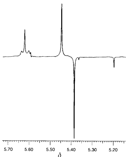
Fig. 10 The partial 400.13 MHz ^1\text{H} NMR spectrum of [(\eta^5\text{-C}_5\text{H}_5)_2\text{Mo}_2(\text{CO})_5(\text{CNMe})] in (\text{CD}_3)_2\text{NDO} at -55^\circ\text{C} . The spectrum was obtained by applying a composite (90_x-240_y-90_x) pulse, delay 1.345 s, and a 90^\circ pulse so that the signal at \delta 5.59 is approximately nulled.
