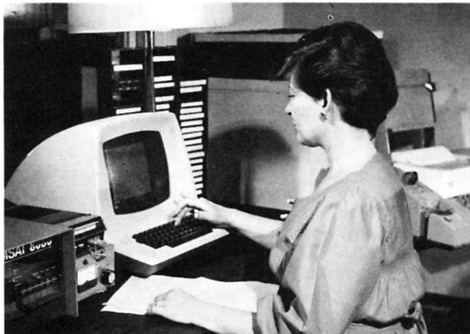
The entire system here is an Imsai 8080 with 24K of memory, ADM-3 terminal, Data Duffer, Teletype... and one efficient secretary.
