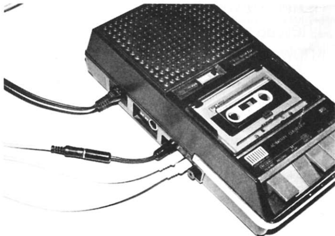
Photo 2. The ungrounding adapter is inserted between the computer and the recorder in the EAR or AUX lines.
