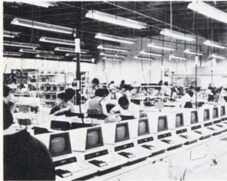
Here's a view of the main part of the PET production department. The front line is brand new PETs that are being checked out with diagnostic programs to make sure they work.
