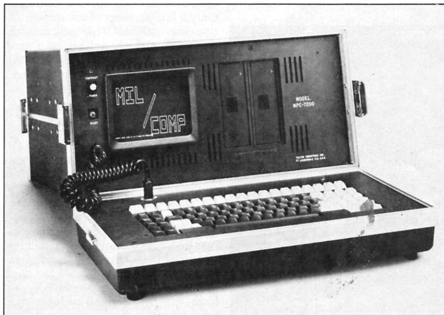
Telcon's Zorba has a 95-key keyboard packed in a 22-pound folding case.
