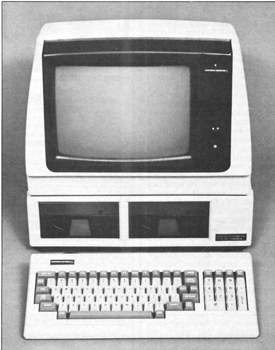
The complete system—computer with two disk drives, 12-inch monitor and detached keyboard.
