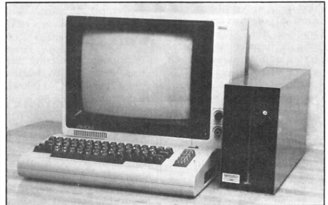
The PEDISK CII is a high-performance disk drive system for the Commodore-64.
