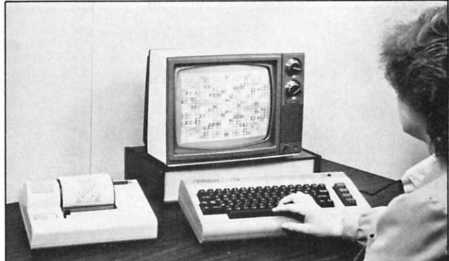
The Alphacom 42, from Alphacom, Inc., is a low-cost, 40-column printer with graphics capabilities for several popular home computers, including those from Commodore, Atari and Texas Instruments.
