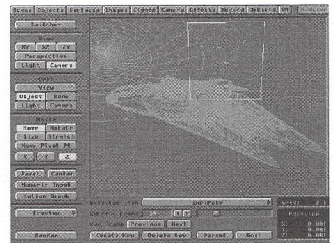
Figure 1: This is what it looked like in layout. Notice the hulking square explosion polygon. It's facing the camera and not oriented in the direction of the ship.
