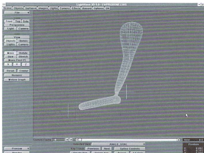
Figure 7: The IK goals set for BoxFoot.LWO are moved and the MetaMation takes effect, transforming the box object into a smooth shape.
