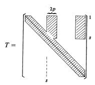
Here s is a point where an eigenvector has converged.
