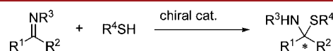
Figure 2. Enantioselective synthesis of N,S -acetals through the addition of thiols to ketimines.
