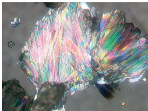
Figure 6. Birefringent crystal of the anhydrous sodium benzoate crystal recrystallized from melt.
