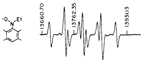
Figure 7. ESR spectrum of the spin adduct of ethyl radical and nitrosodurene obtained during the decomposition of 0.02 M \text{Et}_2\text{Fe}(\text{bpy})_2^+\text{ClO}_4^- and 0.02 M nitrosodurene in THF at 30 °C.
