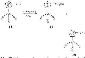
identified by comparing it with an authentic sample of  $(\eta^5-C_5H_4CH_3)Cr(CO)_2NO$ , which was prepared from sodium methylcyclopentadienide in 57% yield following a literature procedure for the parent compound 1.4 The hydrogenolysis of other ketone derivatives of 1 with LiAlH<sub>4</sub>/AlCl<sub>3</sub> has been reported.<sup>4</sup>
