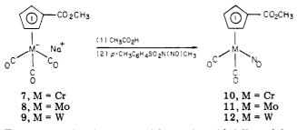
Treatment of anions 7-9 with acetic acid followed by subsequent nitrosylation with N-methyl-N-nitroso-ptoluenesulfonamide produced the respective dicarbonyl nitrosyl derivatives 10 (79%), 11 (12%), and 12 (41%).  $(\eta^5-C_5H_4CHO)Cr(CO)_2NO$  (13) and  $(\eta^5-C_5H_4COCH_3)Cr$ - $(CO)_2NO$  (14) were prepared analogously to compound 10
