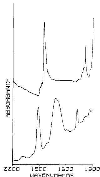
Figure 4. Upper figure: infrared spectrum (Fluorolube mull) of [\text{CpNiCO}]_2 . Lower figure: infrared spectrum of [\text{CpNiCO}]_2 on a DA surface.
