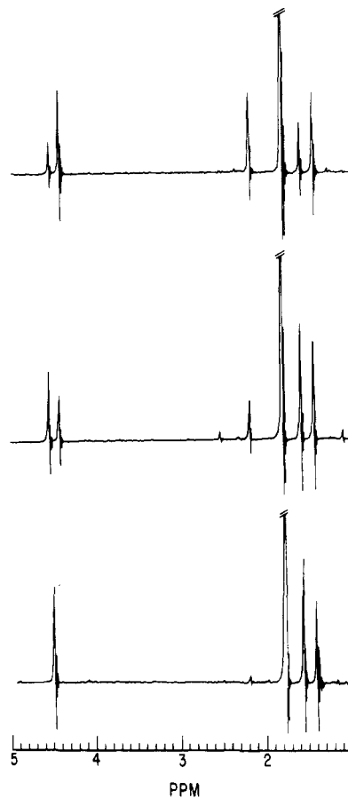
Figure 1. 1 H NMR spectra of a solution of 0.1 M ( p -xylene)-Cr(CO) 3 and 0.12 M (hexamethylbenzene)Cr(CO) 3 in benzene at 0, 105, and 208 h of heating at 170 °C. In addition to resonances of reactive species (see text), peaks at 1.4 and 1.8 ppm represent cyclohexane and (hexamethylbenzene)tricarbonylchromium, respectively.
