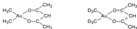
Figure 1. Chemical structures of the dimethyl(2,4-pentanedionato)gold ( 1a ) and the (dimethyl- d 8 )(2,4-pentanedionato)gold ( 1b ) used in these studies.
