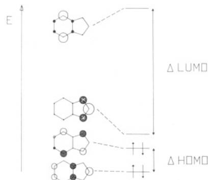
Figure 6. Frontier \pi orbitals and their energy splittings calculated for 1 by the PPP method.
