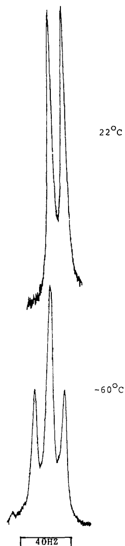
Figure 3. 1 H NMR spectra of 1 in CDCl 3 . The resonances are centered at δ = 1.63 ppm for the doublet and δ = 1.69 ppm for the “triplet”.
