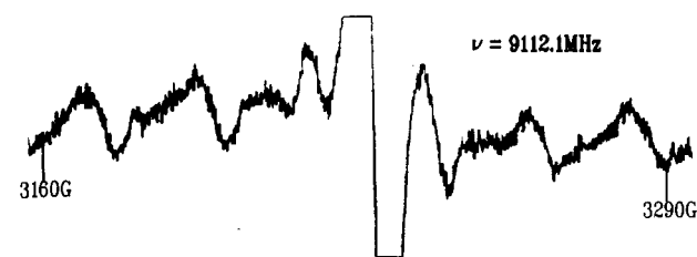
Figure 5. First-derivative EPR spectrum of the \text{Mo}(\text{CO})_5^- radical for B_{0\parallel}X(a^*) in the \text{PPN}^+\text{HMo}(\text{CO})_5^- crystal at 77 K, showing the ^{96,97}\text{Mo} hyperfine manifold.
