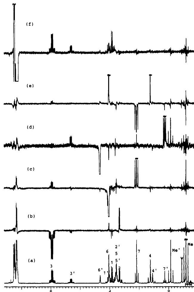
Figure 3. 400-MHz 1 H NMR (a) and NOE difference (b-f) spectra of 2a in CDCl 3 at 25 °C. Selective irradiation was applied at H 3 (b), H 6 (c), H 7 (e), and Ph (f). Overlapping H 2 , H 5 , and H 6 resonances could be assigned by NOE difference spectra irradiating at H 3 , H 4 , and H 4 , respectively. 195 Pt satellites are recognized except for H 2 , H 5 , H 6 , H 6 , and H 6 . W denotes H 2 O.
