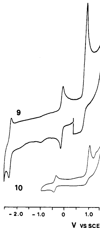
Figure 3. Cyclic voltammograms of 9 (upper trace, -50 °C) and 10 (lower trace, +25 °C) in DME/0.1 M Bu_4NClO_4 , \nu = 0.1 V/s.
