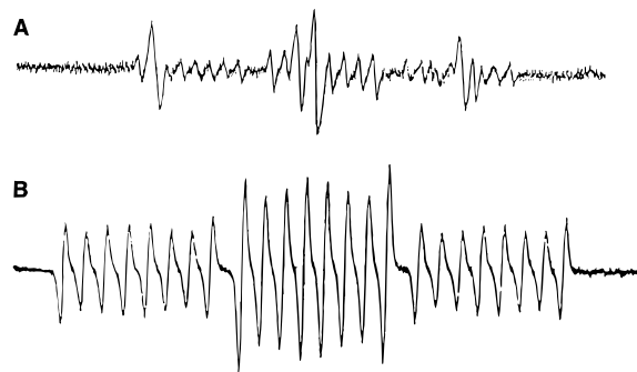
Figure 1. (A) ESR spectrum of the products of the reaction Co(CO) 3 L 2 (1 × 10 -3 M) + DMAD (4 × 10 -3 M) in CH 2 Cl 2 at room temperature. The multiline residual signal near the baseline is caused by a small amount of unreacted Co(CO) 3 L 2 (see (b)). The ESR signal of the products is at least 100 times weaker than that of Co(CO) 3 L 2 at the beginning of the reaction. (B) ESR spectrum of Co(CO) 3 L 2 in THF at 25 °C.
