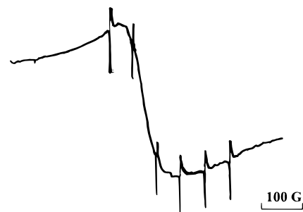
Figure 5. ESR spectrum of (\text{Me}_2\text{SiSiMe}_2)[(\eta^5\text{-C}_5\text{H}_4)\text{Fe}(\text{CO})_2(\mu\text{-CO})_2] ( 1 ) maintained at 145 °C for 45 min.
