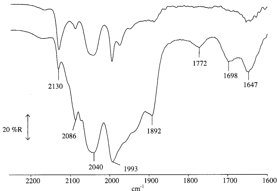
Figure 7. DRIFT difference spectra of the \text{Cr}(2\text{-Me-allyl})_3/\text{SiO}_2(800) catalyst with low CO coverage (above) and after saturating the sample with CO (below). The spectra are relative to the spectrum before CO exposure.
