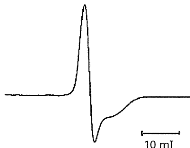
Figure 3. EPR spectrum of [(C_5Me_5)Ir(abpy)Cl]^\bullet- from brief in situ reduction (1 e) of [(C_5Me_5)Ir(abpy)Cl](PF_6) in CH_3CN/0.1 M Et_4NPF_6 at 110 K.
