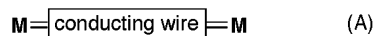
Chart 1. Design Principle of sp-Carbon Molecular Wires [M = organometallic endgroup; A, B, C, D see text]
