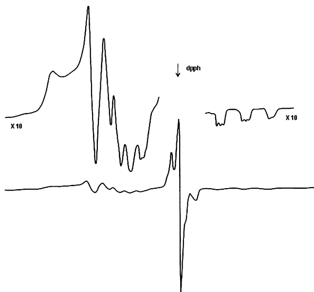
Figure 2. Frozen solution EPR spectrum of a toluene/dichloromethane solution of i -C 3 H 7 Co(DH) 2 py irradiated at 77 K and recorded at 100 K.
