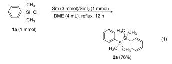
extensive studies concerning different solvents, ratios of  $Sm/SmI_2$ , and reaction temperatures (Table 1), we observed that the best result was obtained when the reaction was conducted
