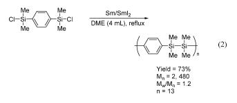
was purified by precipitation from its THF solution by addition of EtOH, followed by freeze-drying. The molecular weight distribution of this polymer was determined by gel permeation chromatography (GPC) calibrated by polystyrene standards with chloroform as the eluent ( $M_n = 2480$ ,  $M_w/M_n = 1.2$ ). This result suggests that the Sm/SmI<sub>2</sub> system is a promising reagent for the construction of a  $\sigma - \pi$  conjugate system of poly(disilanylenephenylene).
