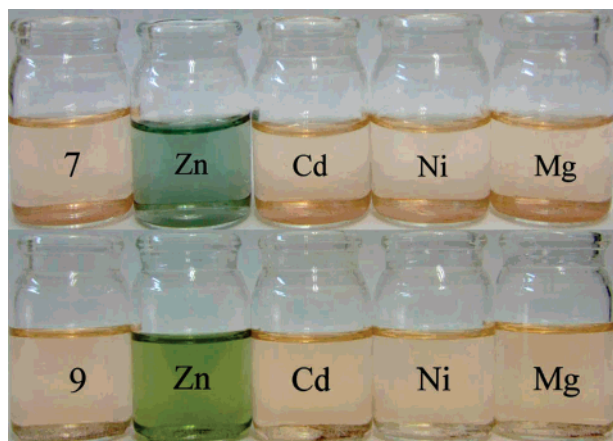
Figure 7. Color changes in \text{CH}_3\text{CN}/\text{CH}_2\text{Cl}_2 solutions of compounds 7 and 9 upon addition of several metal cations tested.
