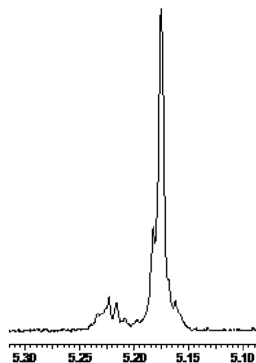
Figure 11. Homonuclear decoupled 1 H NMR spectrum (500 MHz, CDCl 3 , 20 °C) of the methine region of isotactic-enriched PLA (entry 2, Table 3).
