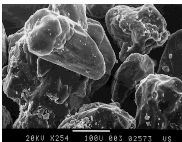
Fig. 11: Scanning electron micrographs of S(+)-ibuprofen, 250fold (a: dry granulated, batch K1; b: spray-coated with the own melt, batch SB 3)
