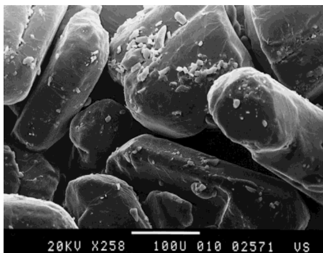
Fig. 8: Scanning electron micrographs of modified recrystallized S(+)-ibuprofen, 250fold (a: batch SEU 2; b: batch SEU 3)
