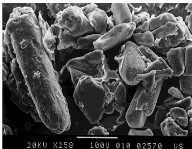
Fig. 12: Scanning electron micrographs of fluid bed granulated S(+)-ibuprofen, 250fold (batch SG 6)
