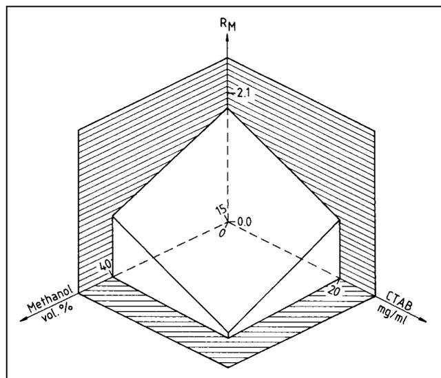
Fig. 1: Effect of methanol and CTAB concentrations in the eluent on the  $R_M$  value of puromycin (compound 17)
