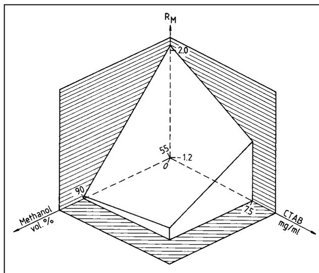
Fig. 2: Effect of methanol and CTAB concentrations in the eluent on the  $R_M$  value of gramicidin (compound 9).
