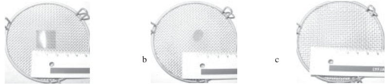
Fig. 4: Swelling of alginate and Carbopol 1832 films in simulated saliva solution: a) initial size; b) alginate film disintegrating after 30 min; c) Carbopol 1382 film expanding after 30 min. The films contain a dye to make them visible in the solution
