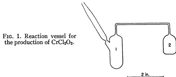
FIG. 1. Reaction vessel for the production of  $\text{CrCl}_2\text{O}_2$ .
