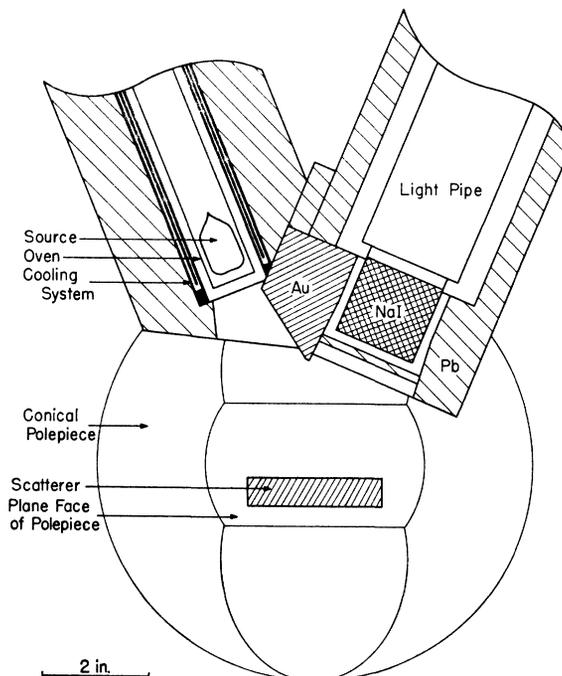
FIG. 4. Experimental arrangement for the precession experiment. The direction of the magnetic field, which was perpendicular to the plane of the drawing, could be reversed.
