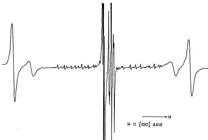
FIG. 1. EPR spectrum of ZnS:Cr<sup>+</sup>, Mn<sup>++</sup>, Fe<sup>3+</sup> with  $H \parallel [100]$  axis.
