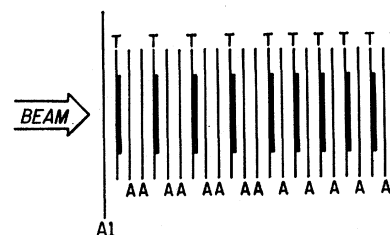
FIG. 1. Sequence of target and degrader foils used in target stack. A1=5.17 mg/cm 2 aluminum foil; T=Target foils, thicknesses listed in Table I; A=2.02 mg/cm 2 aluminum catcher-degrader foils.
