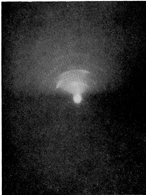
FIG. 7. Electron diffraction of a 37 000-Å film of Nb.
