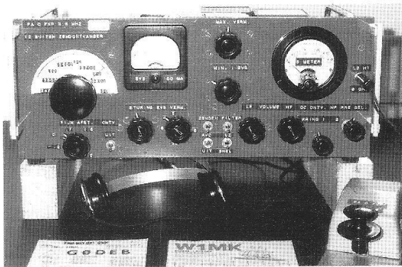
Foto home made 12 tubes OFKP trx 80 m. band.
