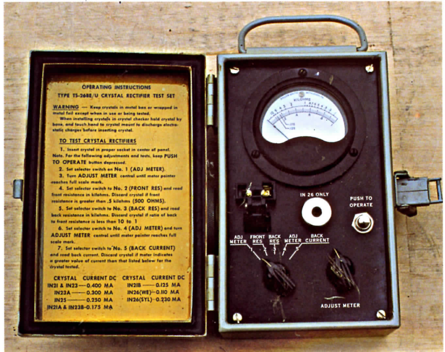
Foto 7: Kristal detector test-apparaat type TS-268E/U Signal Corps US Army
