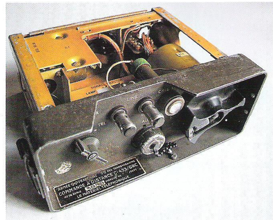
Foto 2 C-433 Remote Control, geopend – dik in de schimmelwerende lak
